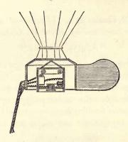
A current passing up by the first wire causes a clockwork apparatus, attached to the camera, to actuate rolls holding the sensitive film in such a manner as to bring a fresh portion of the film behind the lens after an exposure has been made.
